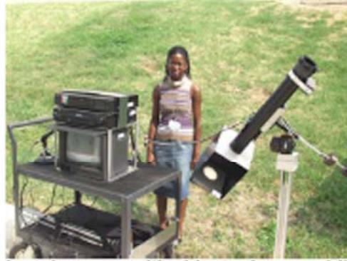
Solar telescope, with videotaping capability, constructed at the Naval Research Laboratory with summer student assistance
