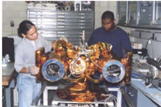
College student interns working at the Naval Research Laboratory participated in the development and testing of a space flight instrument, Global Imaging Monitor of the Ionosphere (GIMI), which was one of several provided by NRL and other DoD agencies, flown on the DoD Space Test Program's ARGOS satellite, launched in February, 1999.
